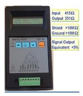
The LCT-01 is a stand-alone portable hand-held device that was especially designed to help technical people immediately analyze the condition of strain-gage based load-cells.
