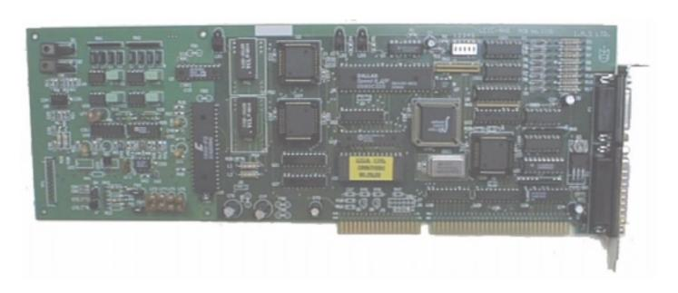
Stand-alone microcomputer-based interface board that was especially designed to fit very fast real-time weighing applications. Requires no other interfacing accessories for the load-cells or the outputs.
